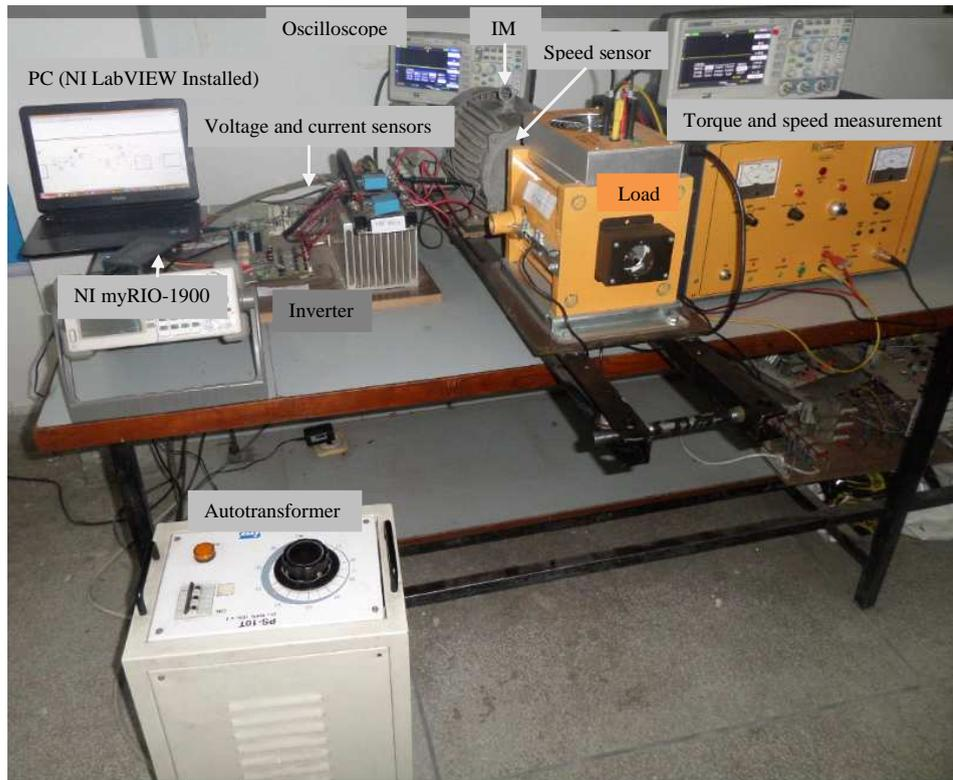
FIGURE 5.13: Experimental setup of an IM drive system.
