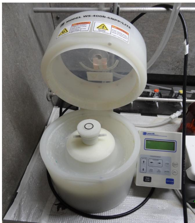
FIGURE 3.4: Spin coater (Laurell WS-650-23NPP) top view. It is used for the growth of thin film using centrifugal principle [168].
