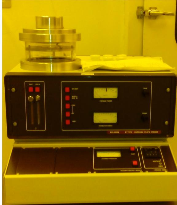
FIGURE 3.1: Plasma etcher used to clean substrate prior to fabrication.
