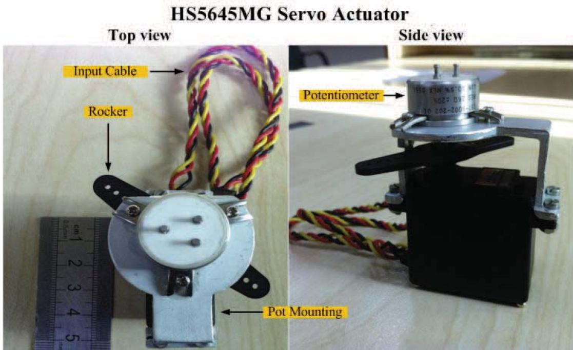
FIGURE A.5: External feedback acquisition mechanism
