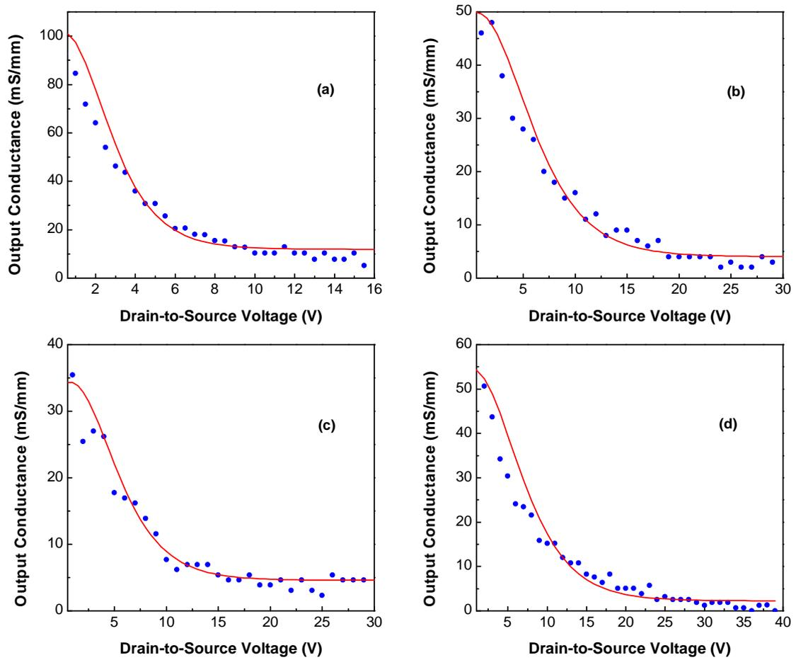
FIGURE 4.3: Experimental (●) and simulated (—) output conductance as function of gate and drain biasing of submicron SiC MESFETs (a)  $0.7 \mu\text{m}$  gate length device, (b)  $0.6 \mu\text{m}$  gate length device, (c)  $0.5 \mu\text{m}$  gate length device and (d)  $0.4 \mu\text{m}$  gate length device.
