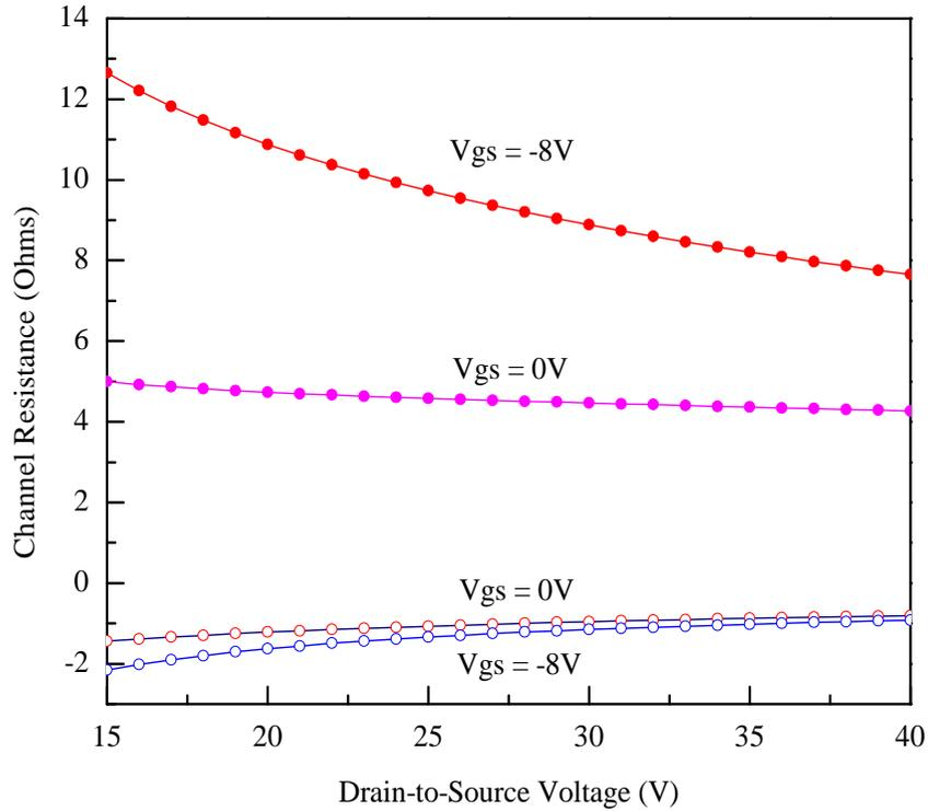
FIGURE 5.10: Channel resistance,  $R_i$  of a  $0.4\mu\text{m}$  SiC MESFET. Open circles ( $\circ$ ) represent values of  $R_i$  attained from the conventional approach whereas, solid circles ( $\bullet$ ) show simulated values of  $R_i$  using the proposed model.
