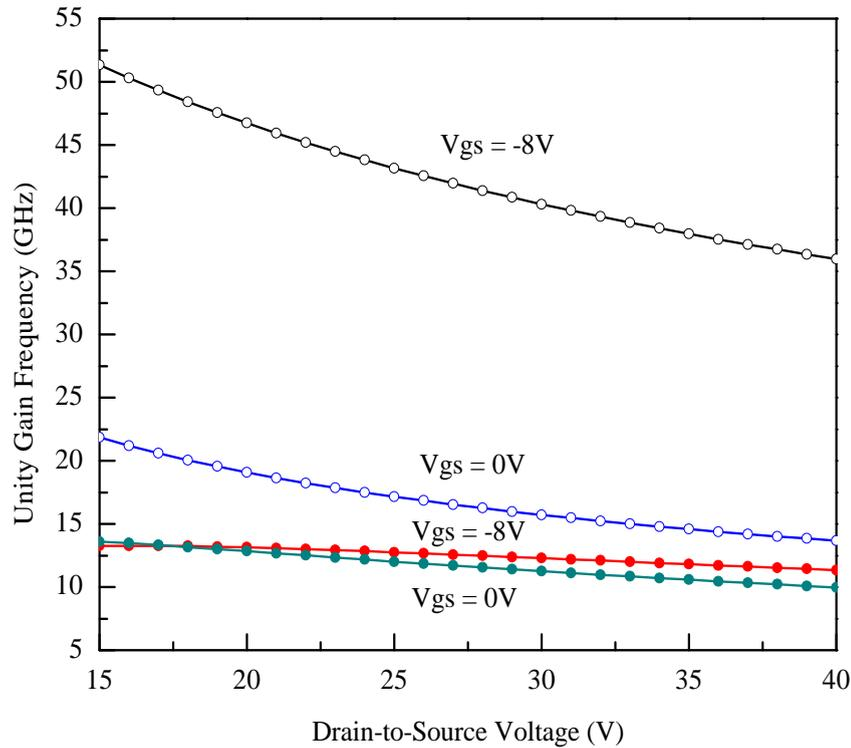
FIGURE 5.11: Unity gain frequency,  $f_T$  of a  $0.4\mu\text{m}$  SiC MESFET. Open circles ( $\circ$ ) represent values of  $f_T$  attained from the conventional approach whereas, solid circles ( $\bullet$ ) show simulated values of  $f_T$  using the proposed model.
