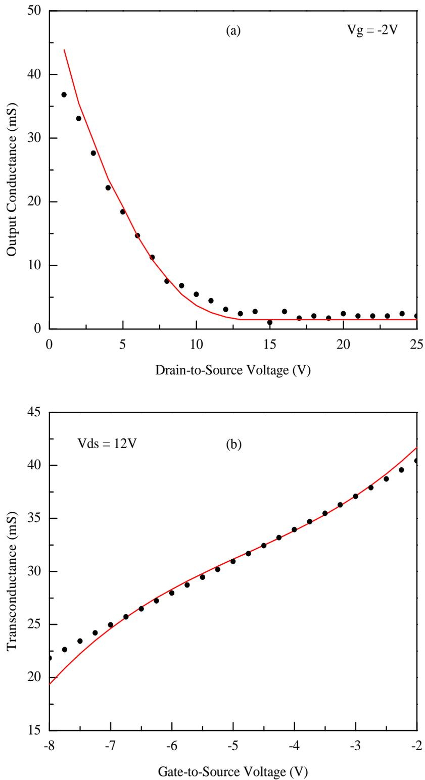
FIGURE 3.10: Modeled (—) and measured (●) (a) output conductance and (b) transconductance of a submicron SiC MESFET.
