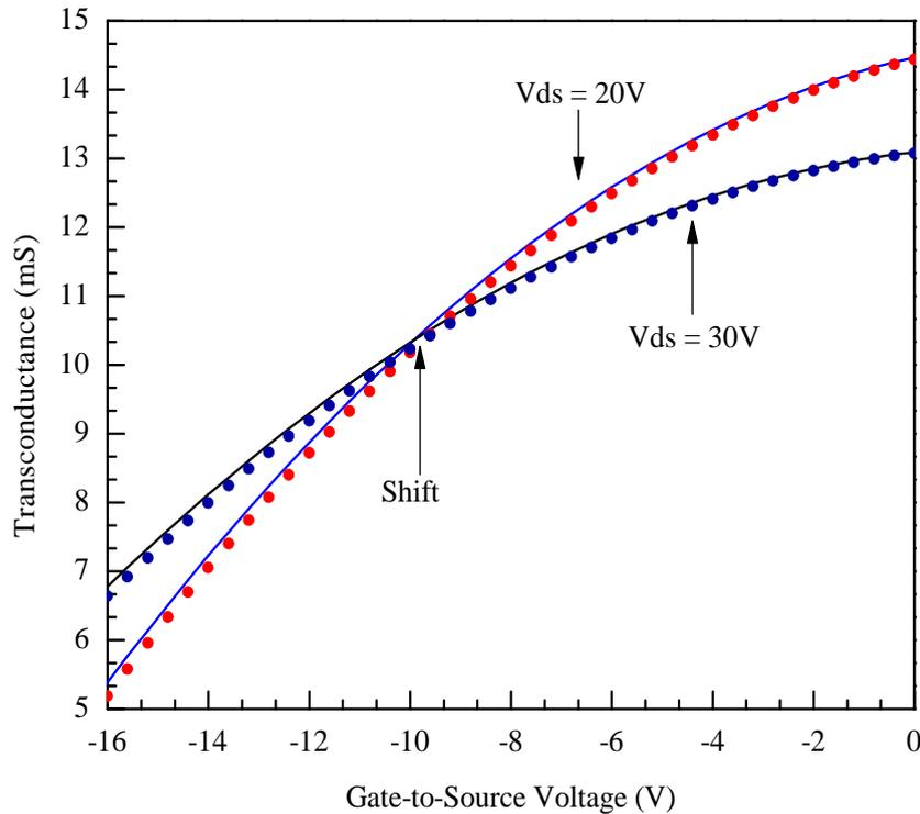
FIGURE 5.3: Transconductance of a submicron SiC MESFET. (—) represents a plot achieved using Eq. 5.15 and (•) represent differentiation of observed  $I - V$  characteristics with respect to  $V_{gs}$ . Point 'shift' represents biasing voltage where the Schottky barrier gate starts performing relatively poor compared to lower biasing voltages.
