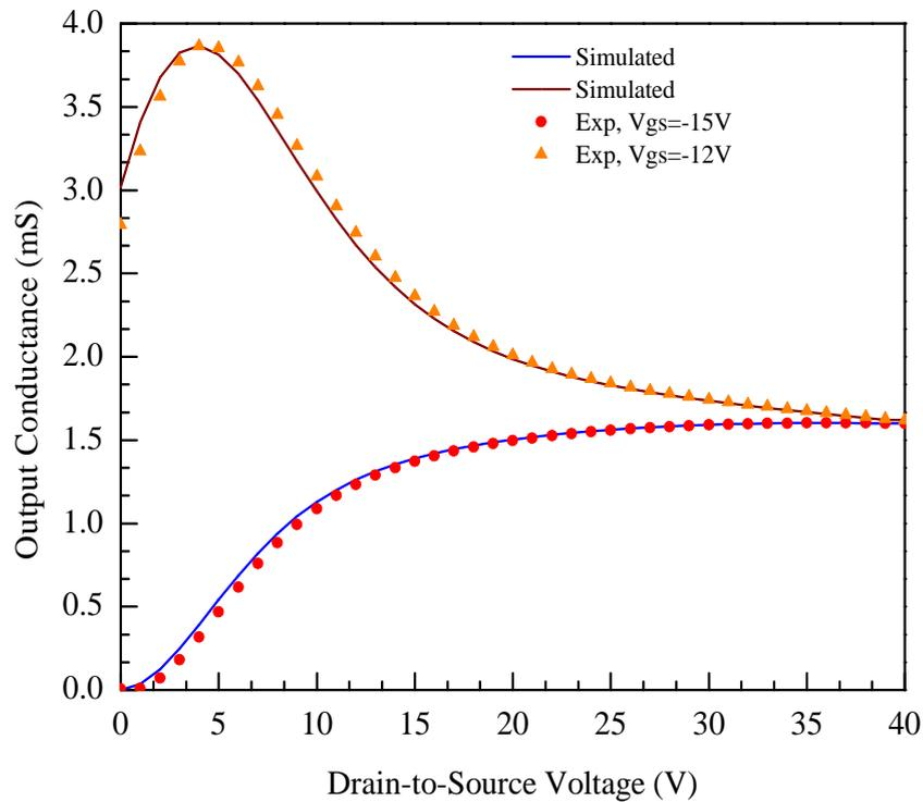
FIGURE 5.4: Output conductance of a submicron SiC MESFET. Plot exhibits that the output conductance which was concave upwards changed to concave downwards with changing gate biasing.
