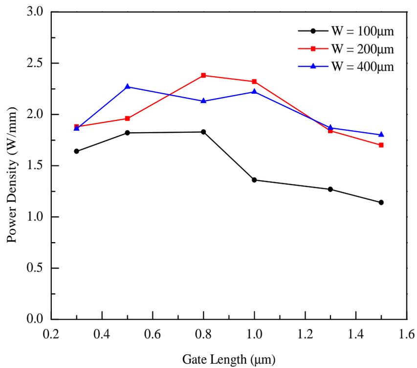
FIGURE 2.3: Power density as a function of  $L_g$  and  $W$ .
