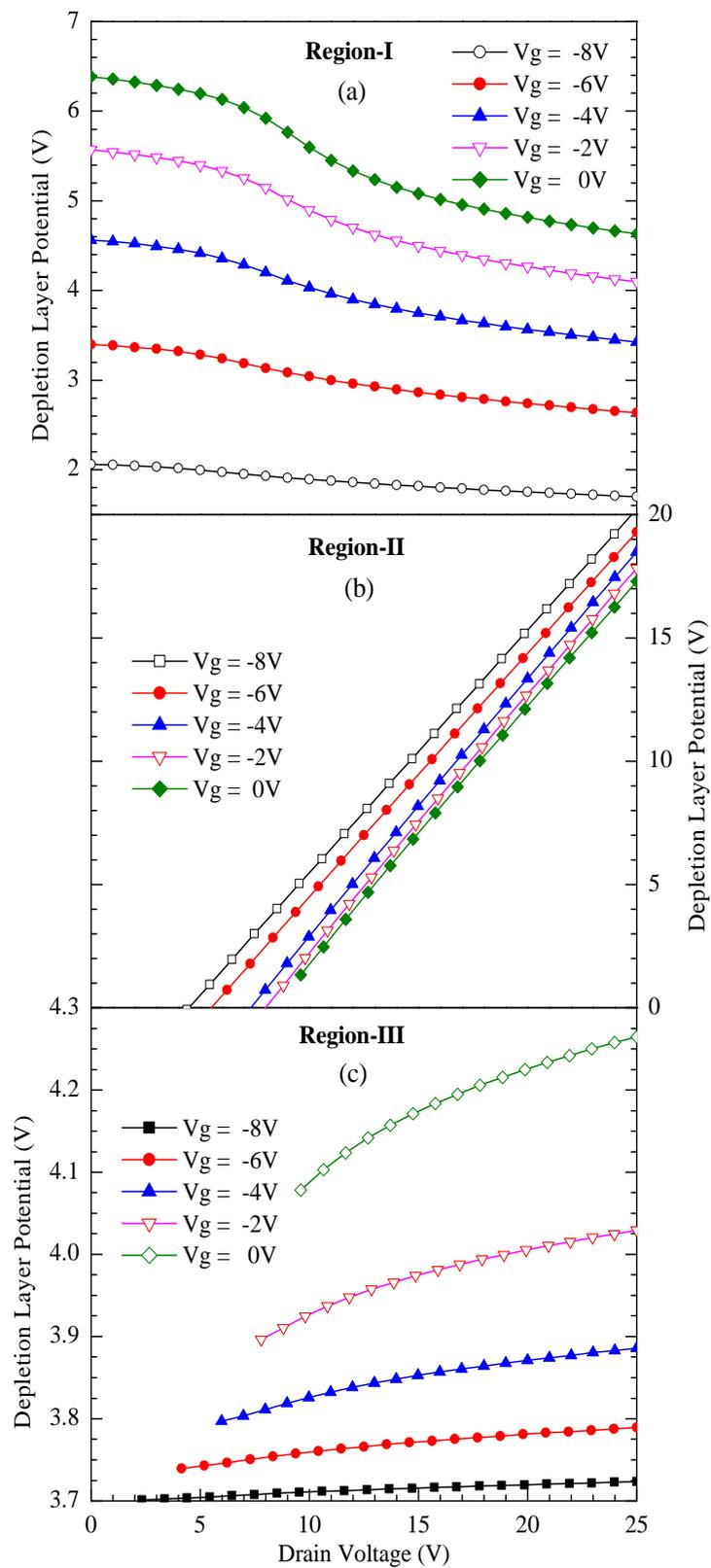
FIGURE 3.4: Depletion layer potential underneath the Schottky barrier gate of a submicron SiC MESFET.
