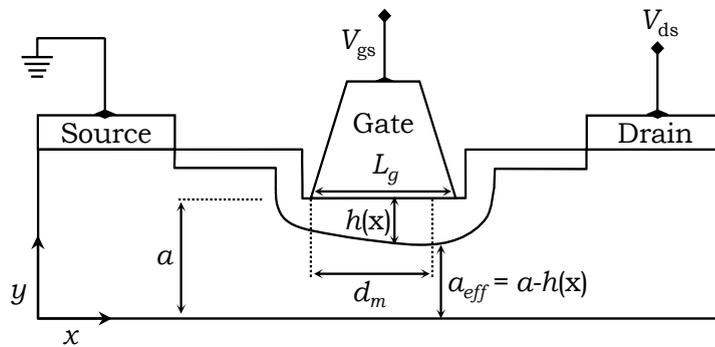
FIGURE 4.1: Cross-sectional view of a SiC MESFET.
