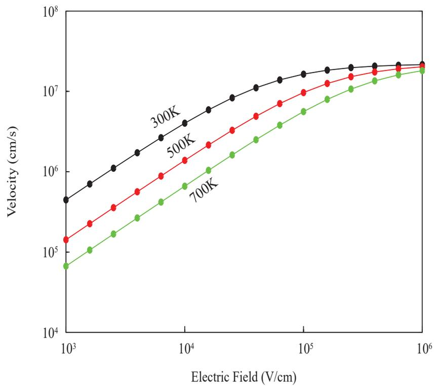
FIGURE 1.2: Velocity as a function of electric field and temperature.
