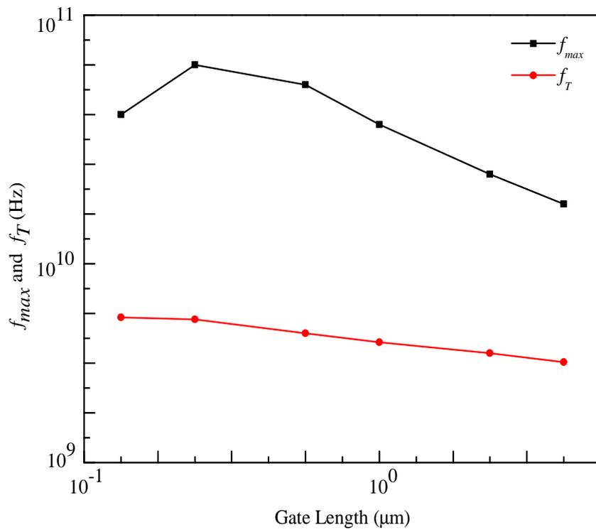
FIGURE 2.2:  $f_{max}$  and  $f_T$  as a function of  $L_g$ .
