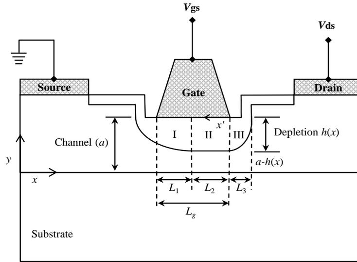
FIGURE 3.1: An operating submicron SiC MESFET with three distinct depletion layer regions underneath Schottky barrier gate.
