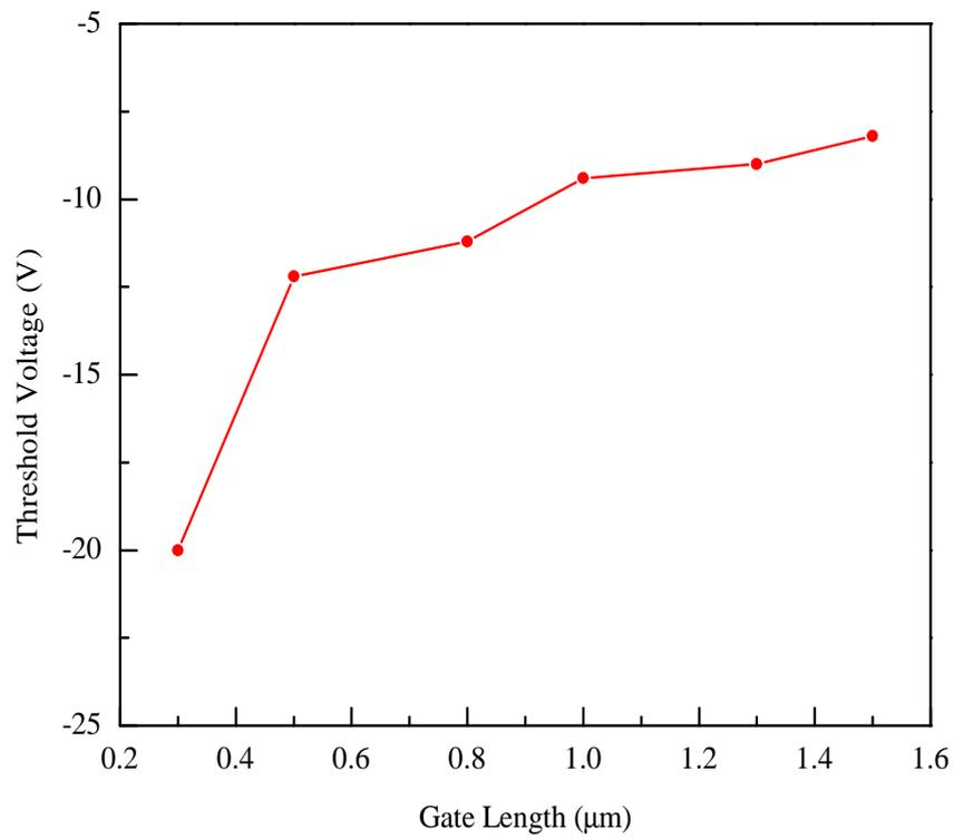
FIGURE 2.5:  $V_T$  as a function of  $L_g$ .
