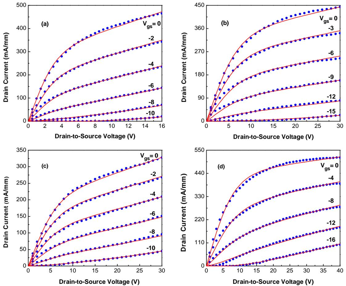
FIGURE 4.2: Experimental ( $\bullet$ ) and simulated ( $-$ ) output characteristics of submicron SiC MESFETs (a)  $0.7 \mu\text{m}$  gate length device, (b)  $0.6 \mu\text{m}$  gate length device, (c)  $0.5 \mu\text{m}$  gate length device and (d)  $0.4 \mu\text{m}$  gate length device.
