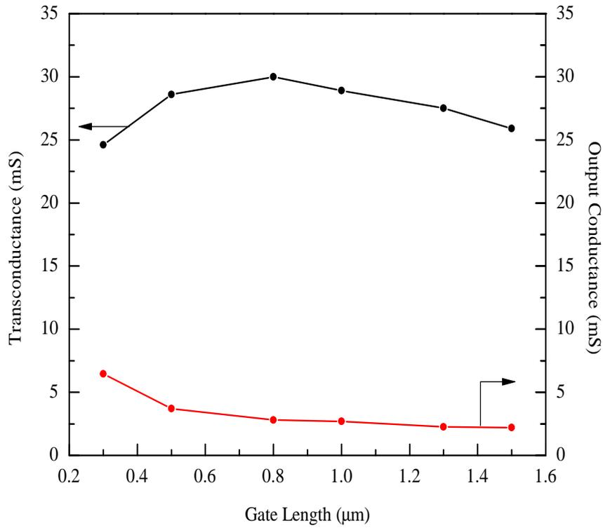
FIGURE 2.1:  $g_m$  and  $g_d$  as function of  $L_g$ .
