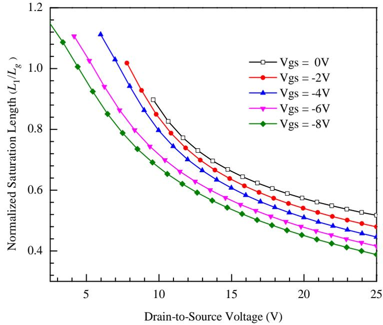
FIGURE 3.7: Shows shifting of saturation length  $L_1$  towards source side of the gate after the onset of current saturation in a SiC MESFET.
