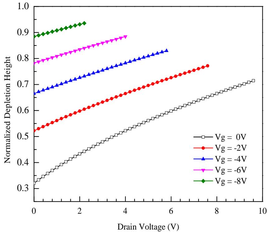
FIGURE 3.3: Variation in Schottky barrier depletion before the onset of current saturation for a submicron SiC MESFET.
