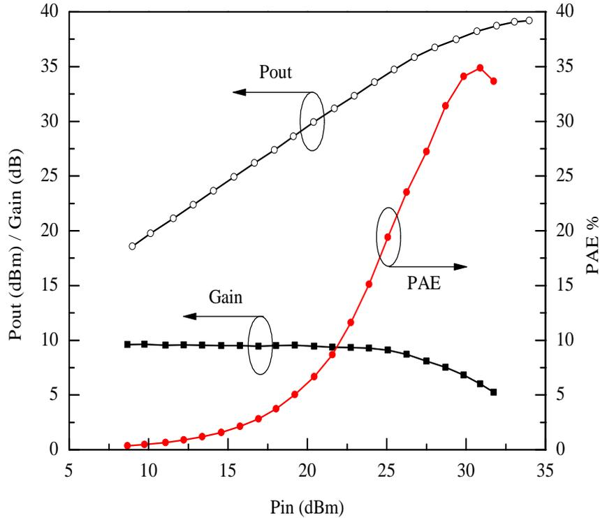
FIGURE 1.6: Power performances measurement at 2 GHz of a 4H-SiC MESFET.
