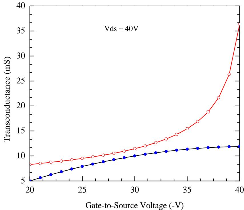
FIGURE 5.9: AC transconductance,  $g_m$  of a  $0.4\mu\text{m}$  SiC MESFET. Open circles (○) represent values of  $g_m$  attained from the conventional approach whereas, solid circles (●) show simulated values of  $g_m$  using the proposed model.
