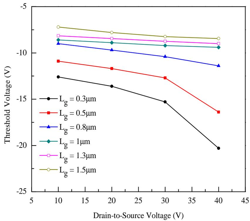
FIGURE 2.6:  $V_T$  as a function of  $V_{ds}$  and  $L_g$ .
