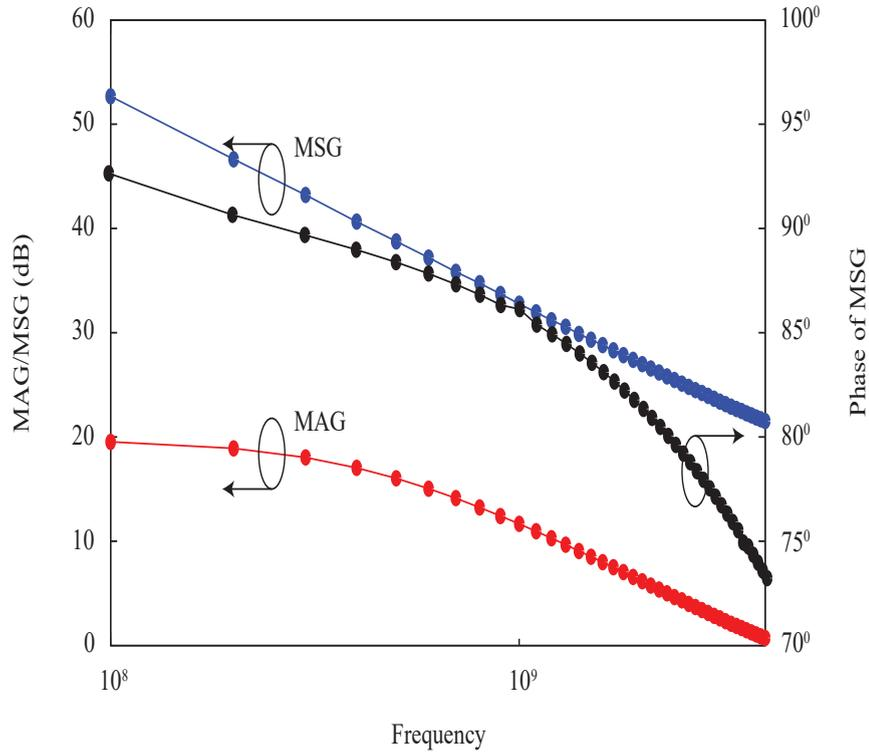
FIGURE 1.5: Plot for MAG, MSG and the phase of MSG for SiC MESFET.
