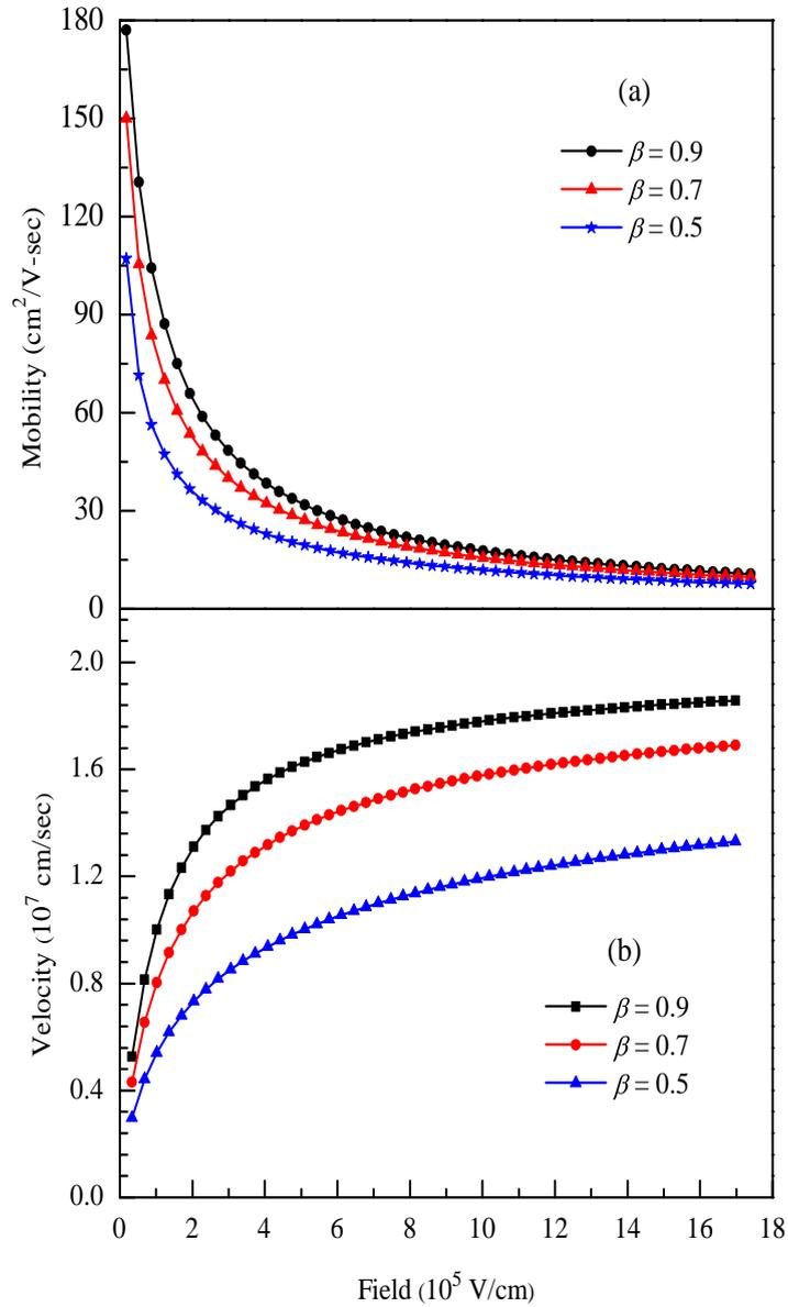
FIGURE 3.2: Field dependent (a) mobility and (b) velocity of a SiC MESFET.
