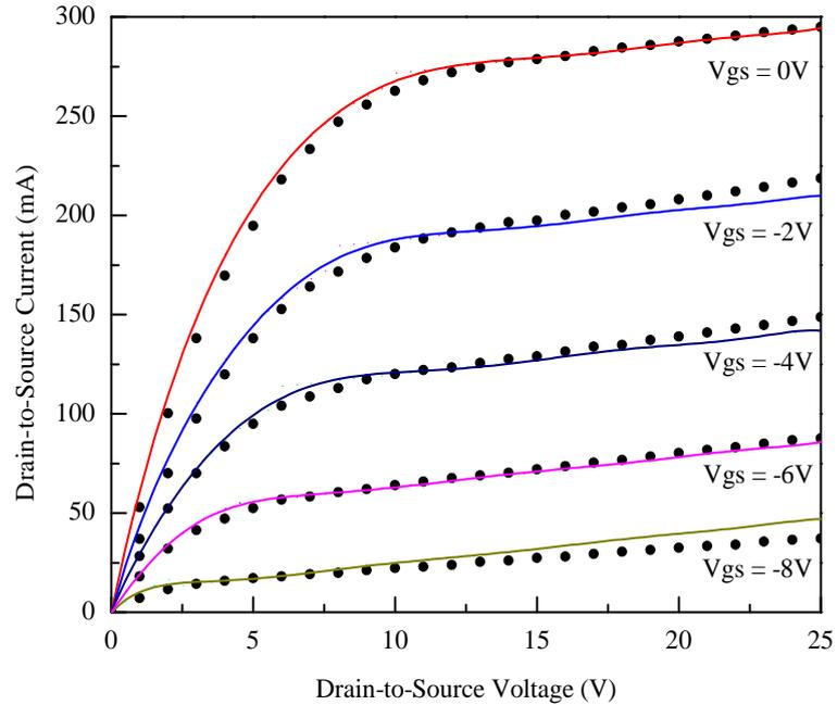
FIGURE 3.5: Modeled (—) and measured (●) output characteristics of a submicron SiC MESFET.
