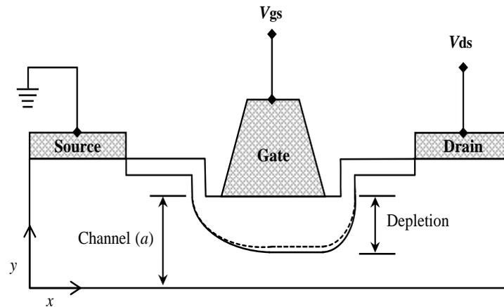
FIGURE 3.8: A cross-sectional view of an operating SiC MESFET where a dotted line shows reduction in gate depletion layer with increased drain biasing.
