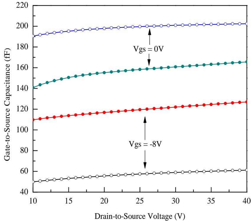
FIGURE 5.5: Gate-to-source capacitance,  $C_{gs}(V_{ds}, V_{gs})$  of a  $0.4\mu\text{m}$  SiC MES-FET. Open circles ( $\circ$ ) represent values of  $C_{gs}$  attained from the conventional approach whereas, solid circles ( $\bullet$ ) show calculated  $C_{gs}$  from the proposed model.
