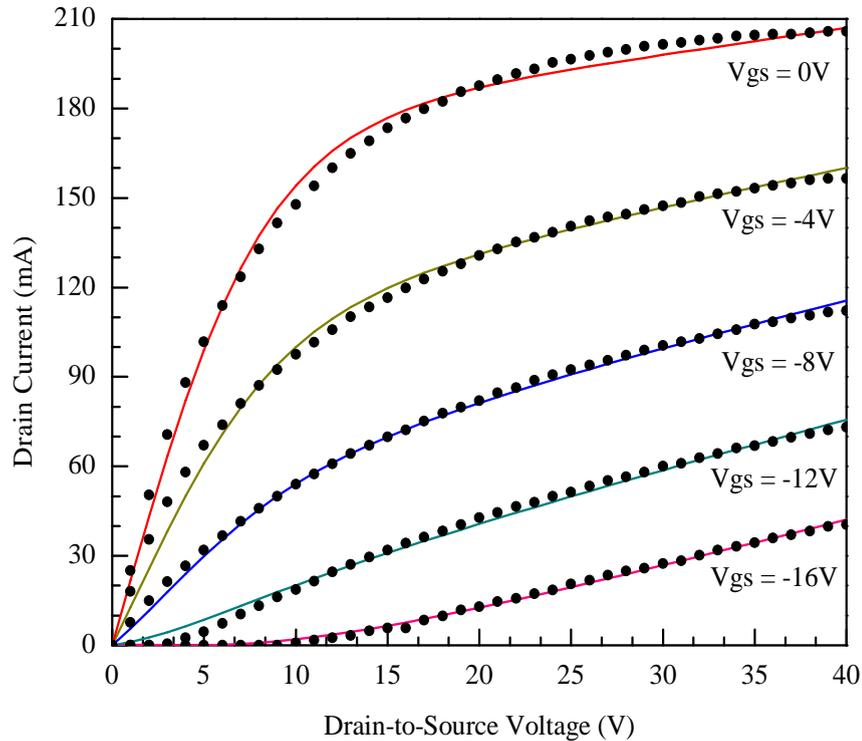
FIGURE 5.2: Simulated (—) using Eq. 5.14 and experimental (●) output characteristics of a  $0.4\mu\text{m}$  SiC MESFET.
