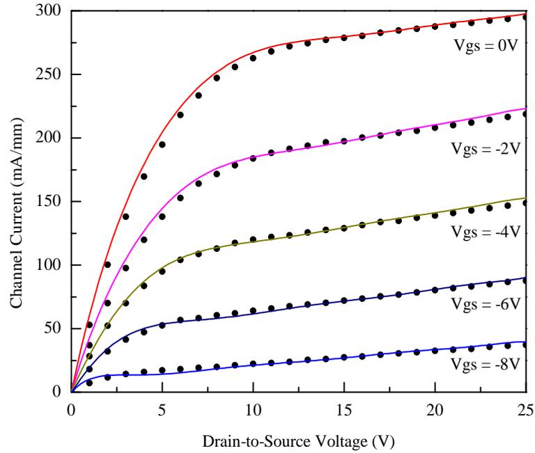
FIGURE 3.9: Output characteristics of a submicron SiC MESFET: measured (●) and modeled (—) with proposed depletion layer modification technique.
