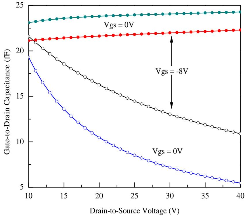
FIGURE 5.6: Gate-to-drain capacitance,  $C_{gd}(V_{ds}, V_{gs})$  of a  $0.4\mu\text{m}$  SiC MESFET. Open circles ( $\circ$ ) represent values of  $C_{gd}$  attained from the conventional approach whereas, solid circles ( $\bullet$ ) show calculated  $C_{gd}$  from the proposed model.
