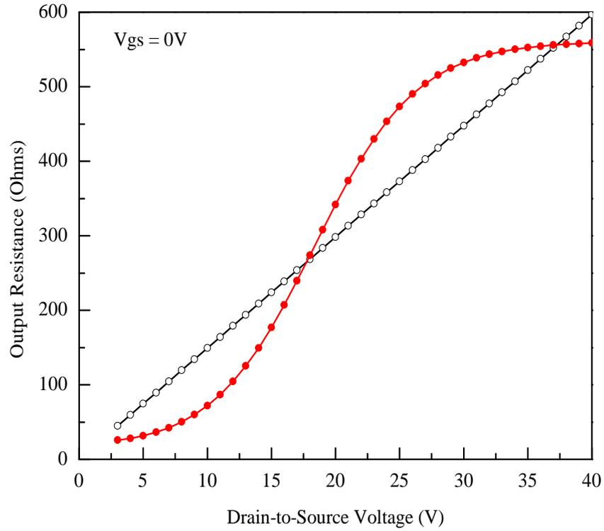
FIGURE 5.12: Output resistance,  $r_0$  of a  $0.4\mu\text{m}$  SiC MESFET. Open circles ( $\circ$ ) represent values of  $r_0$  attained from the conventional approach whereas, solid circles ( $\bullet$ ) show simulated values of  $r_0$  using the proposed model.
