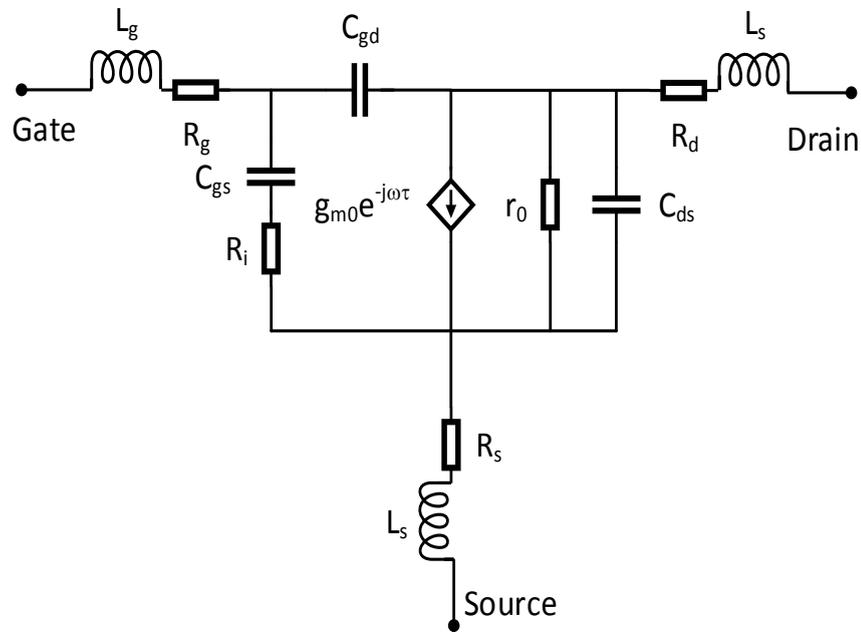
FIGURE 5.13: AC equivalent circuit of a SiC MESFET.
