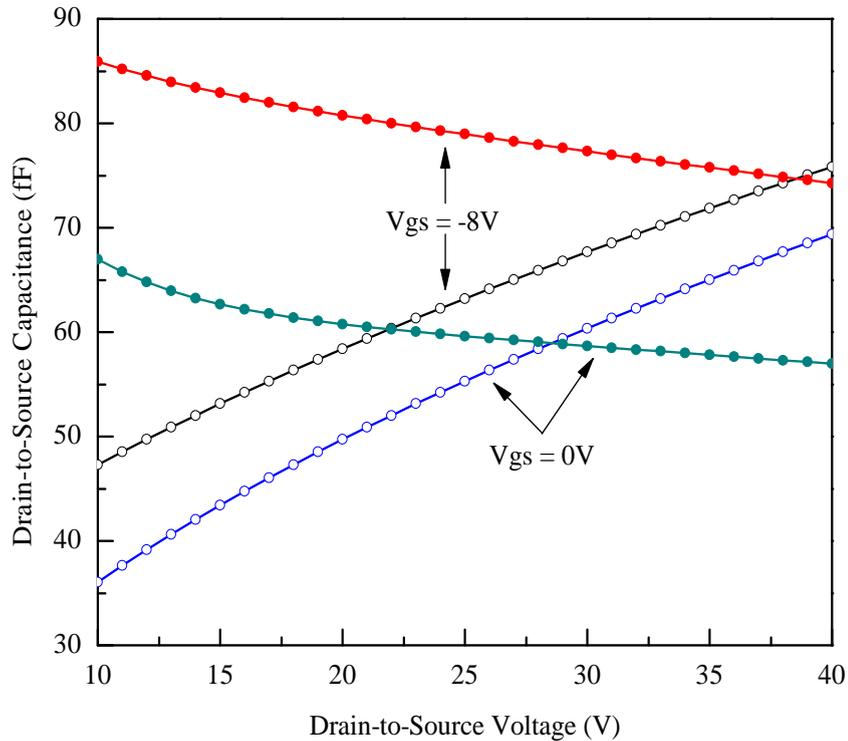
FIGURE 5.7: Drain-to-source capacitance,  $C_{ds}(V_{ds}, V_{gs})$  of a  $0.4\mu\text{m}$  SiC MES-FET. Open circles ( $\circ$ ) represent values of  $C_{ds}$  attained from the conventional approach whereas, solid circles ( $\bullet$ ) show calculated  $C_{ds}$  from the proposed model.
