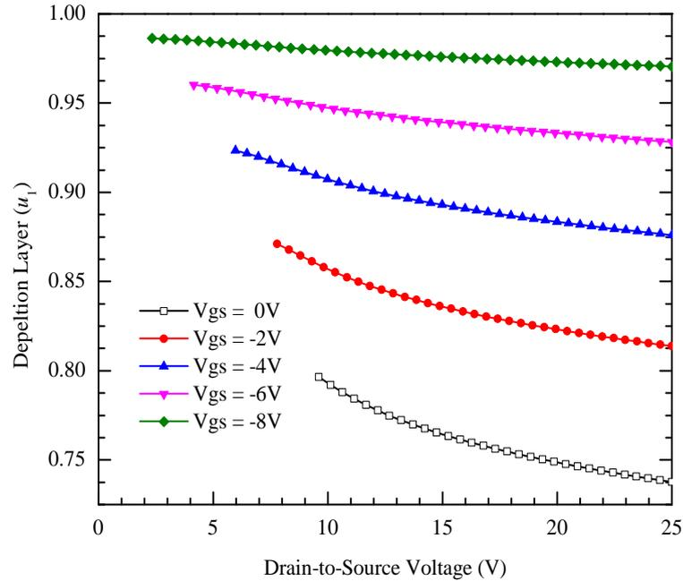
FIGURE 3.6: Variation in depletion layer after the onset of current saturation in a SiC MESFET.
