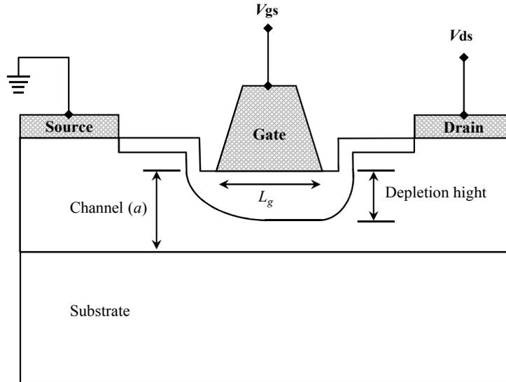
FIGURE 1.3: Cross-sectional view of the schematic of a MESFET.
