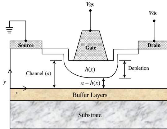
FIGURE 5.1: Cross-sectional view of a SiC MESFET.
