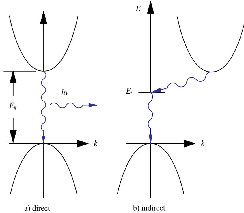
FIGURE 2.4: Direct and indirect transition in semiconductor (a) Direct transition with emission of photon, (b) Indirect transition via defect level.
