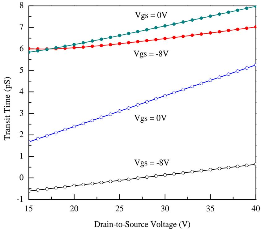
FIGURE 5.8: Transit time,  $\tau$  of a  $0.4\mu\text{m}$  SiC MESFET. Open circles ( $\circ$ ) represent values of  $\tau$  attained from the conventional approach whereas, solid circles ( $\bullet$ ) show simulated values of  $\tau$  using the proposed model.
