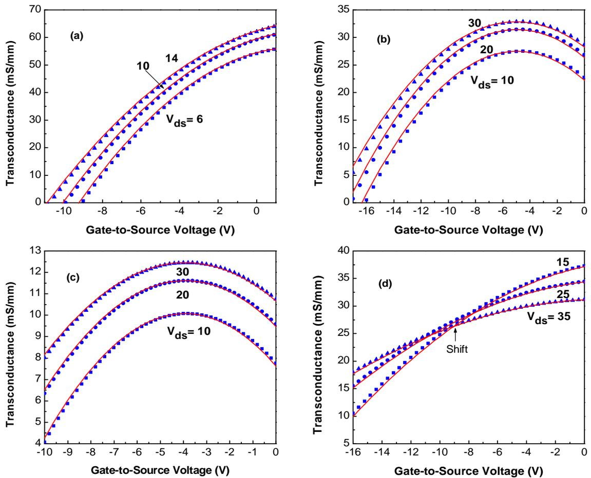
FIGURE 4.4: Experimental ( $\bullet$ ) and simulated ( $-$ ) transconductance as function of gate and drain biasing of submicron SiC MESFETs (a) 0.7  $\mu\text{m}$  gate length device, (b) 0.6  $\mu\text{m}$  gate length device, (c) 0.5  $\mu\text{m}$  gate length device and (d) 0.4  $\mu\text{m}$  gate length device.
