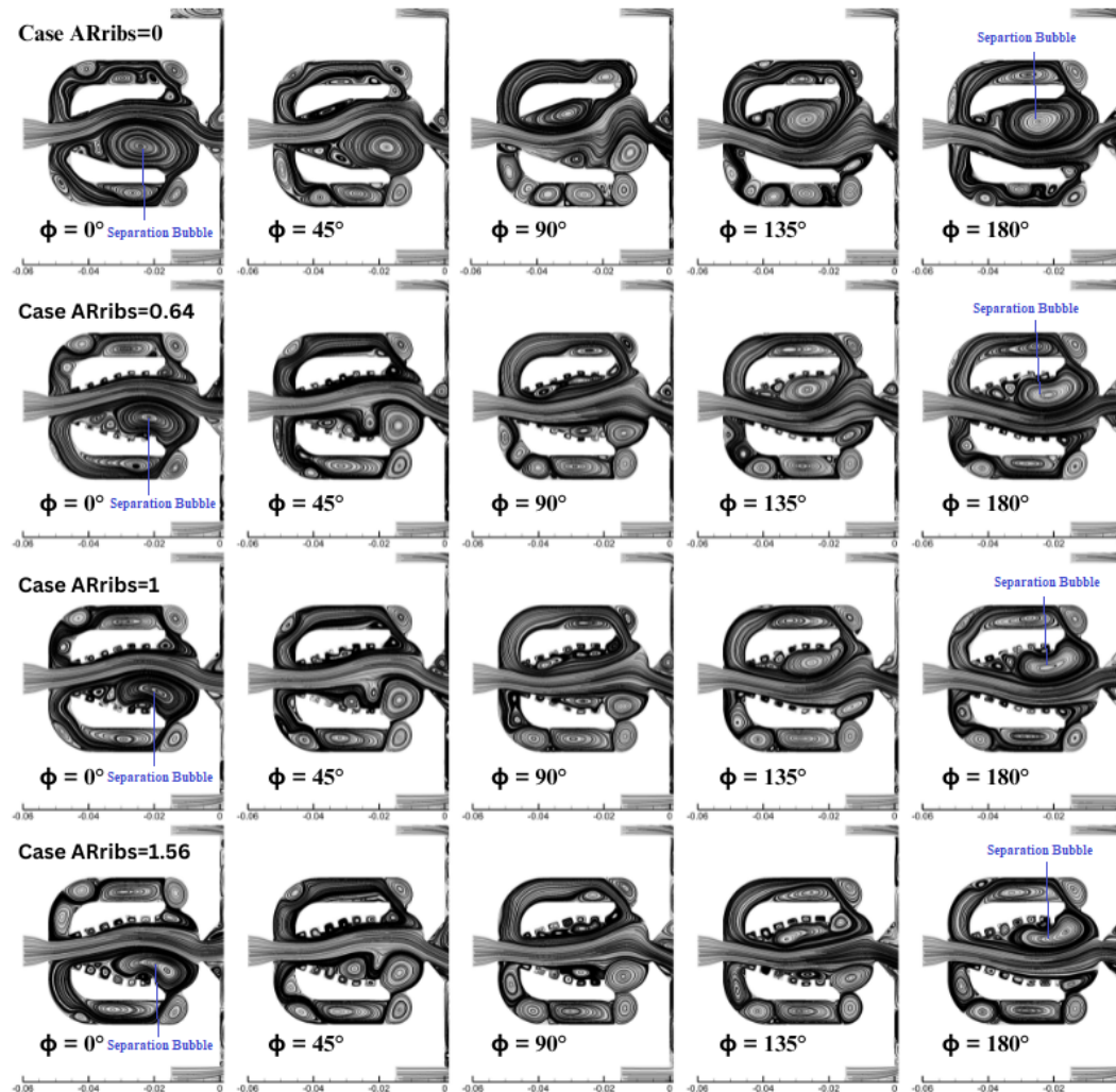
FIGURE 4.2: Streamline plots highlighting the effect of ribs on the formation of separation bubbles at different phase angles for different aspect ratios of ribs placed over the Coanda surface
