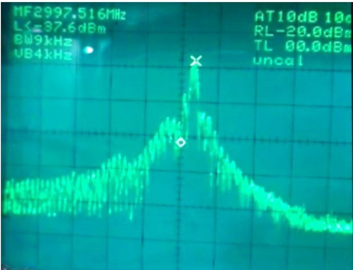
FIGURE 6.22: Frequency Spectrum of Magnetron forward Power after Injection Pulling/ Locking
