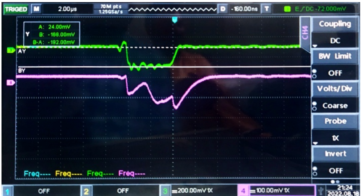
FIGURE 6.14: Time domain Scope signal measurement of Reflected(purple) and Forward signal(green) in Magnetron twining case
