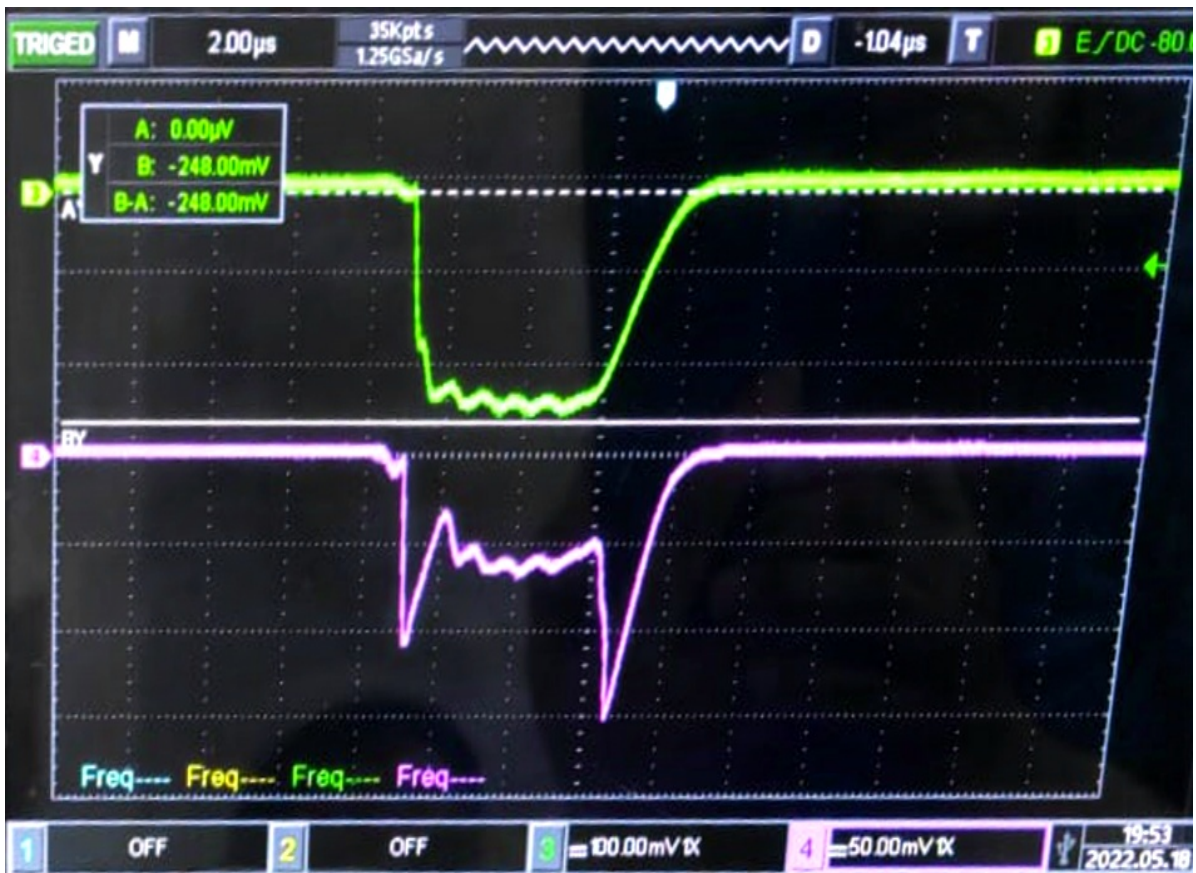
FIGURE 6.23: Forward(green) and reflected signal(purple) from the directional coupler for minimum reflection
