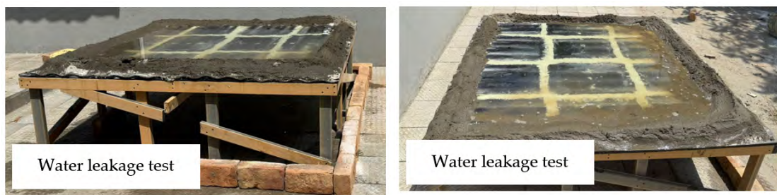
FIGURE 5.16: Water leakage testing of recycled plastic corrugated prototype slabs test
