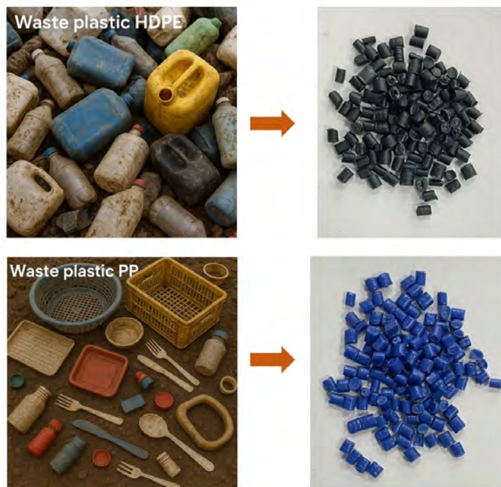
FIGURE 5.1: Recycling of Waste plastic to form pellets of HDPE and PP
