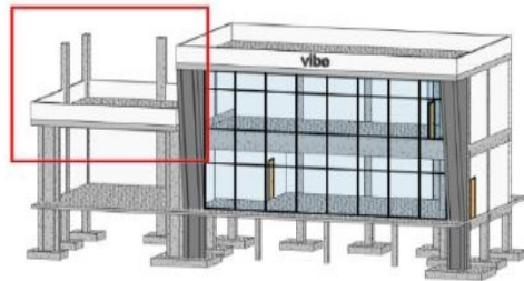
d. Column C-4 shows continuity till 1st floor structure plan.
