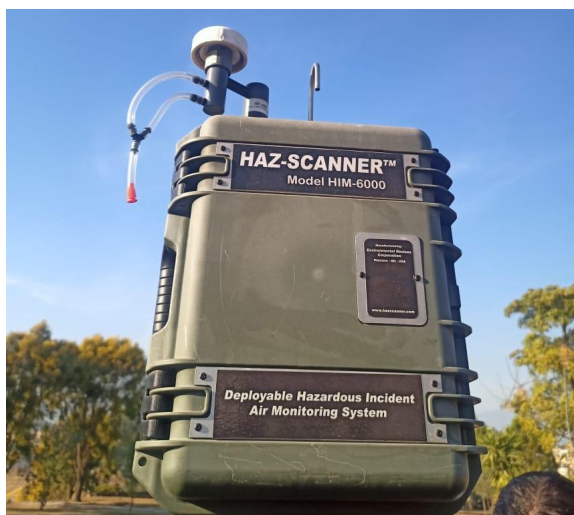
FIGURE 3.12: Air monitoring system for collecting smog air samples
