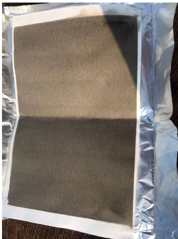
FIGURE 3.13: Particulate collection by quartz microfiber filters
