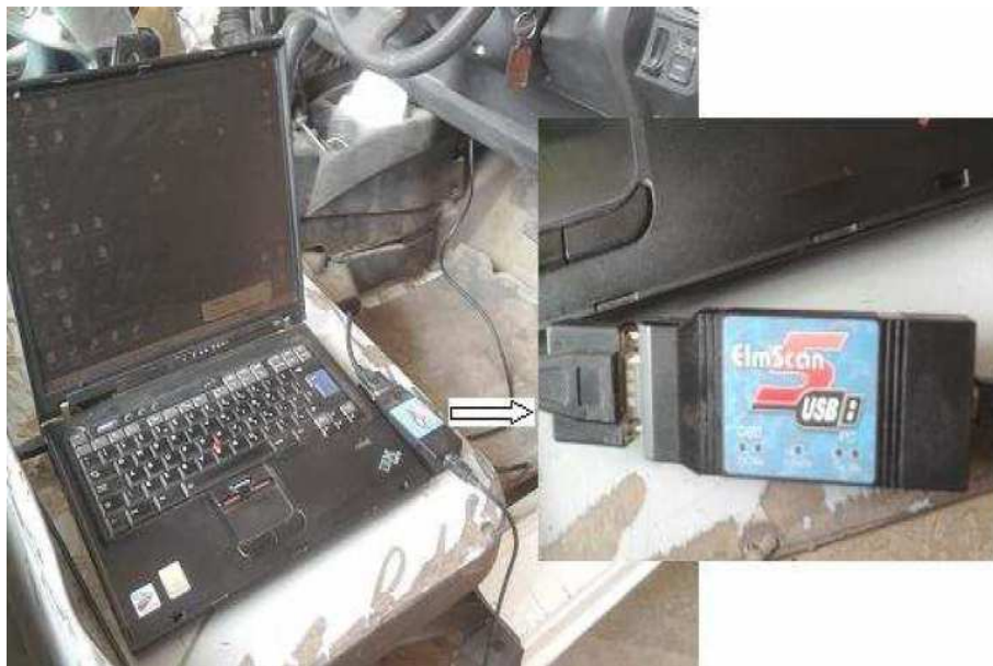
Figure-5.12 Data acquisition through OBD-II connector
