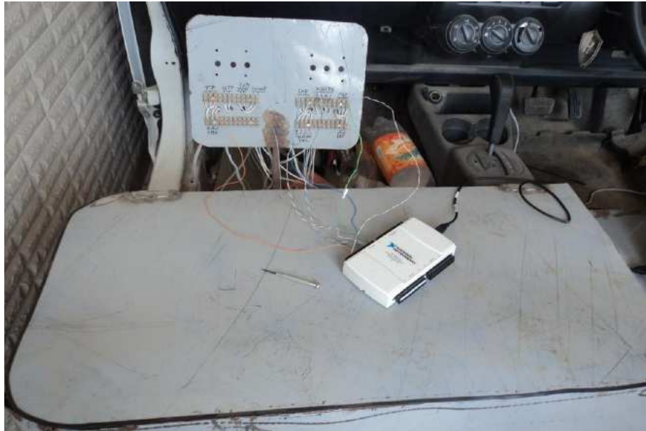
Figure-5.11 NI card used for data acquisition
