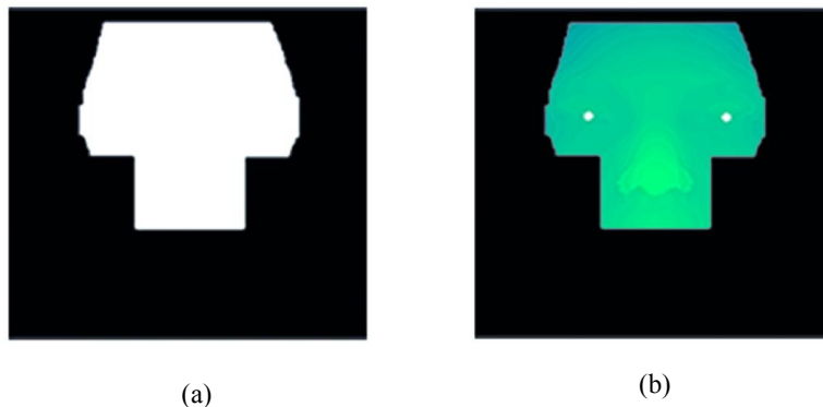
Fig. 5.3 (a) Binary mask for segmentation of expression invariant area (b) expression invariant area of the face for example subject from FRGC v2.0
