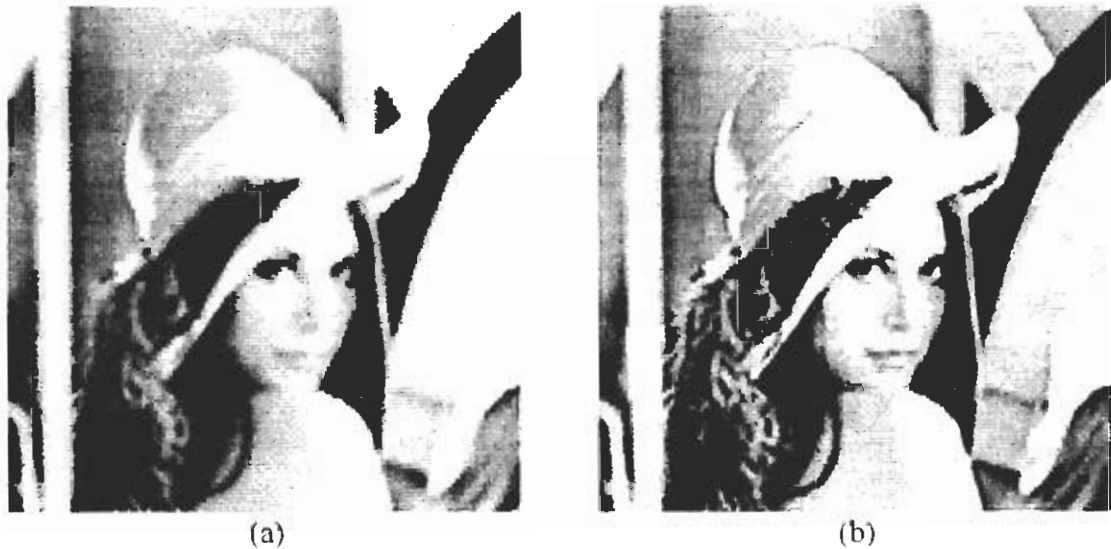
Figure 5.6 Blind image deconvolution degraded images with quantization noise, having SNR of 20db, using neural networks based on nonlinear ARMA model. a) Degraded image of 'Lena' , b) Restored 'Lena' image.
