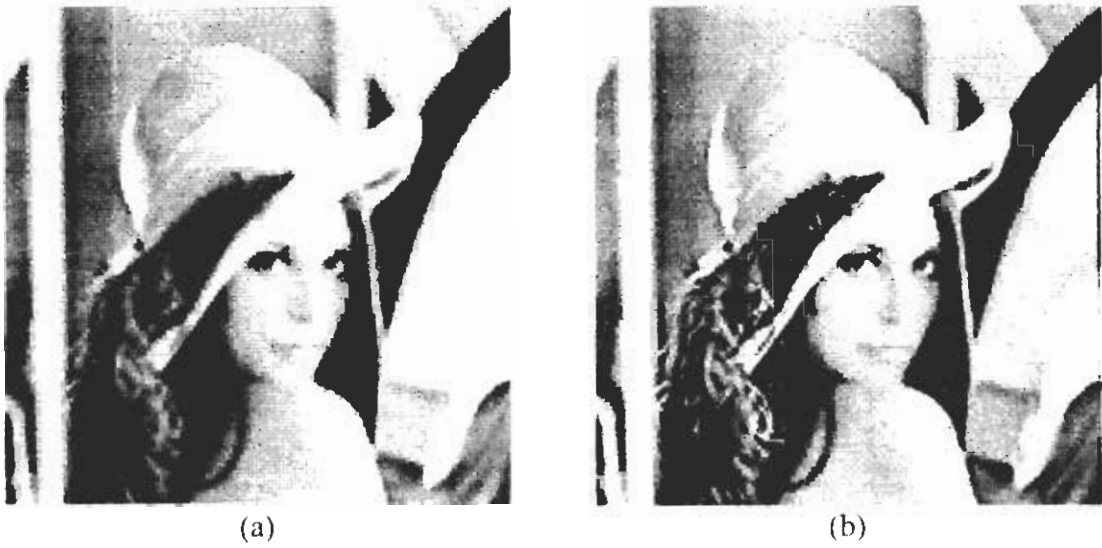
Figure 6.4 Blind image deconvolution of degraded images with AWGN having 30db SNR using neural networks based on space-variant linear ARMA model. a) Degraded image of 'Lena', b) restored Image.
