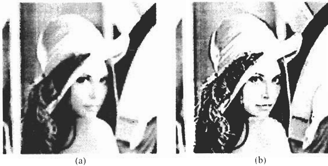
Figure 6.2 Blind deconvolution of images degraded with linear and space-invariant process, having SNR of 30db, using neural networks based on space-variant linear ARMA model. a) Degraded image of 'Lena' with 30db SNR and small quantization noise, b) Restored image of 'Lena'
