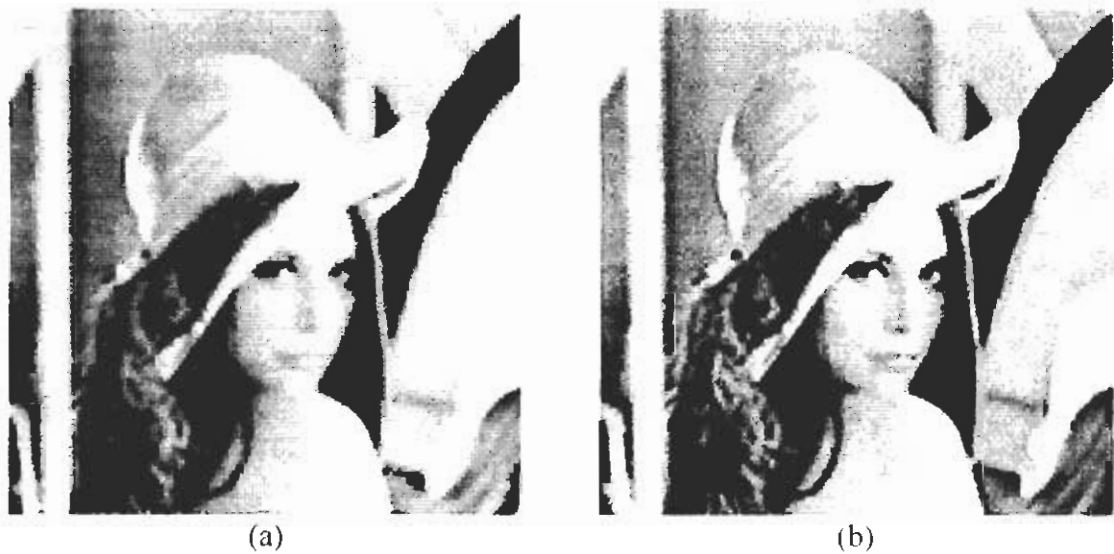
Figure 5.4 Blind image deconvolution of nonlinearly degraded images with AWGN having SNR of 20db using neural networks based on linear AR model. a) Degraded image of 'Lena', b) 'Lena' image restored using neural network.
