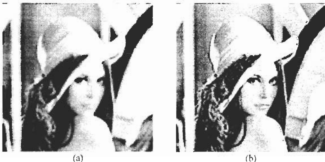
Figure 5.8 Blind image deconvolution of nonlinearly degraded images with AWGN, having 20db SNR, using neural networks based on nonlinear ARMA model. a) Degraded image of 'Lena', b) Restored image of 'Lena'.
