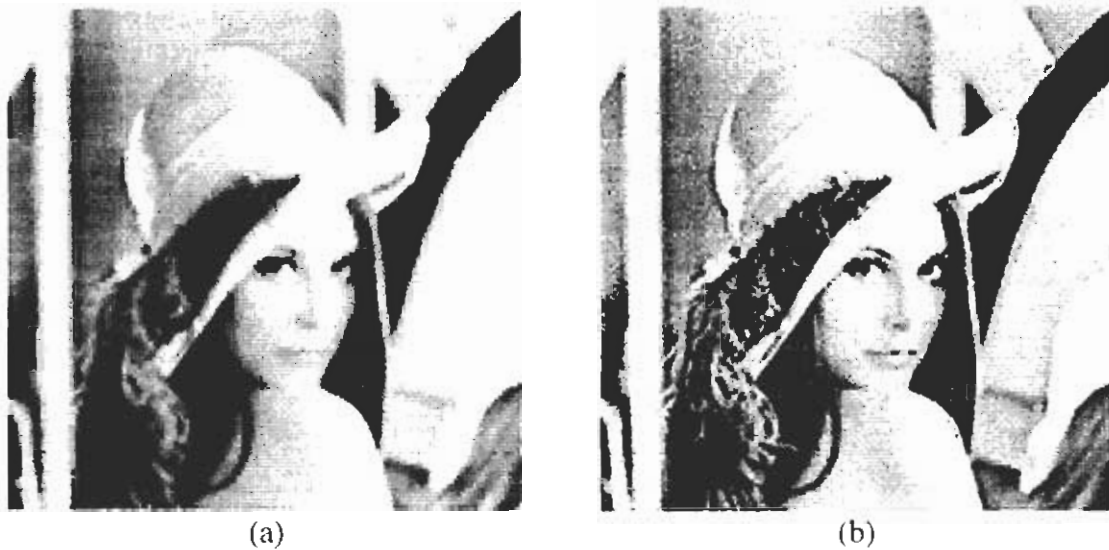
Figure 5.7 Blind image deconvolution of nonlinearly degraded images with AWGN, having SNR of 30db, using neural network based on nonlinear ARMA model. a) Degraded image of 'Lena', b) Restored image of 'Lena'
