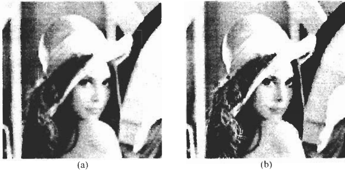
Figure 6.10 Blind deconvolution of images degraded by a linear and space-variant process with AWGN using space-variant neural network approach. a) Degraded image of 'Lena' having SNR= 20db. b) Restored image of 'Lena'
