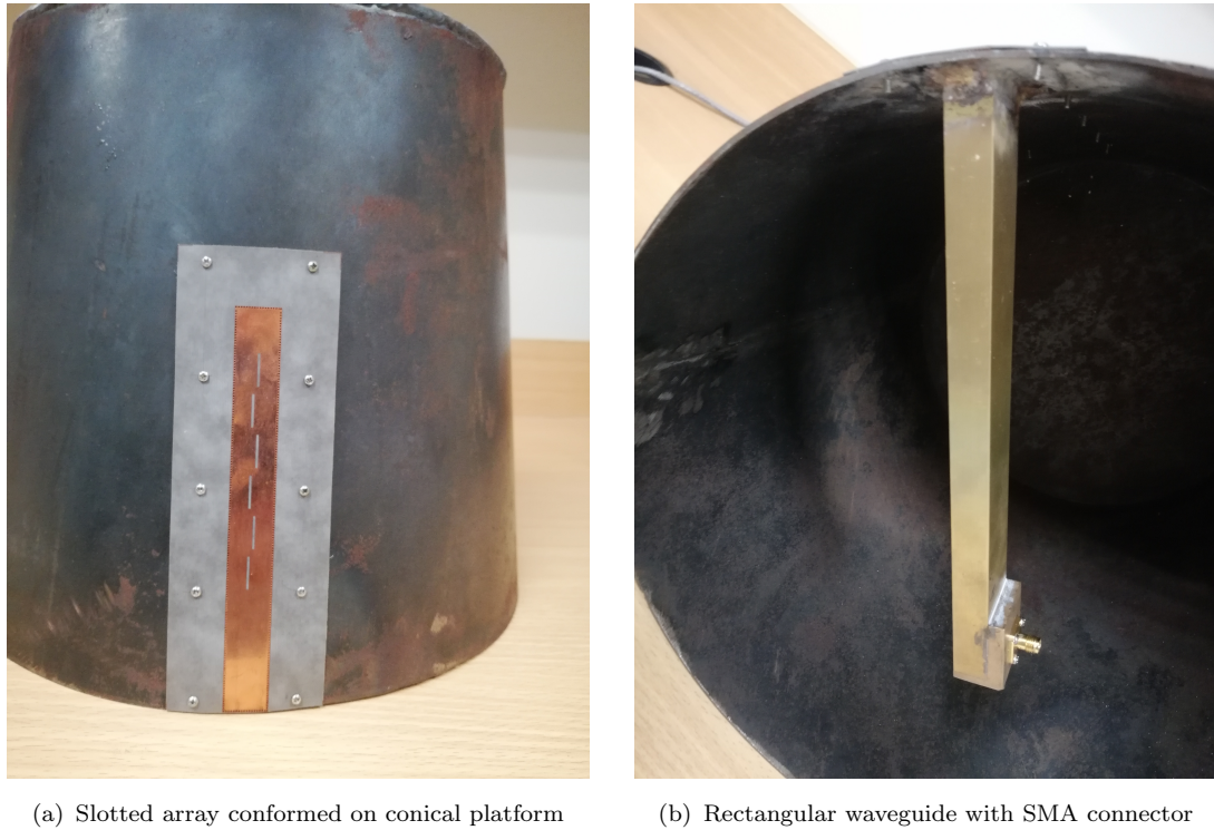
FIGURE 7.11: Prototype of the fabricated nose-cone conformal slot array antenna.
