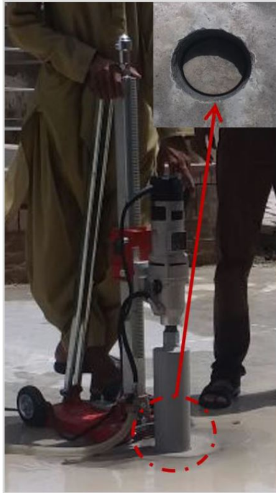
FIGURE 6.7: Core drilling test assembly.
