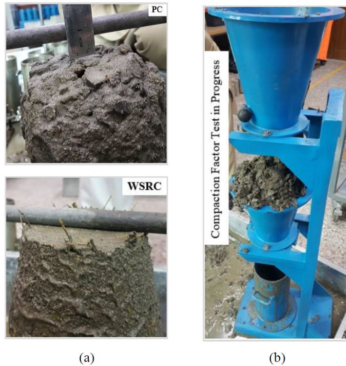
FIGURE 6.3: Workability tests (a) Slump value and (b) Compaction factor test of PC and WSRC mix
