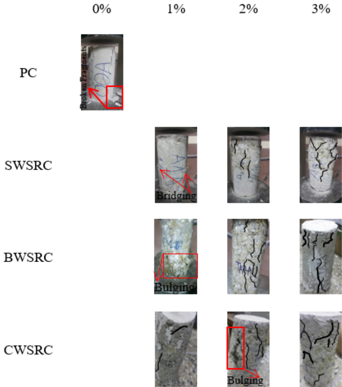
FIGURE 3.4: Tested cylinder specimens of PC and WSRC with varied treatment and fibre content under compressive loading.
