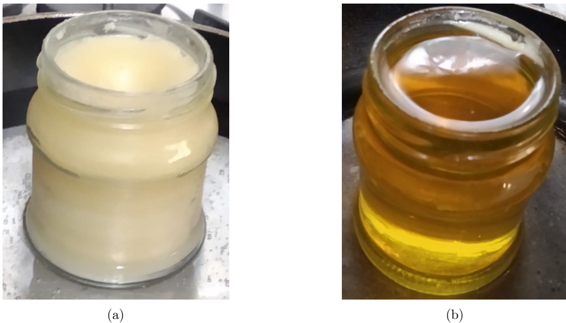
FIGURE 3.6: (a) Solid and (b) liquid phases of stearic acid ( PCM).
