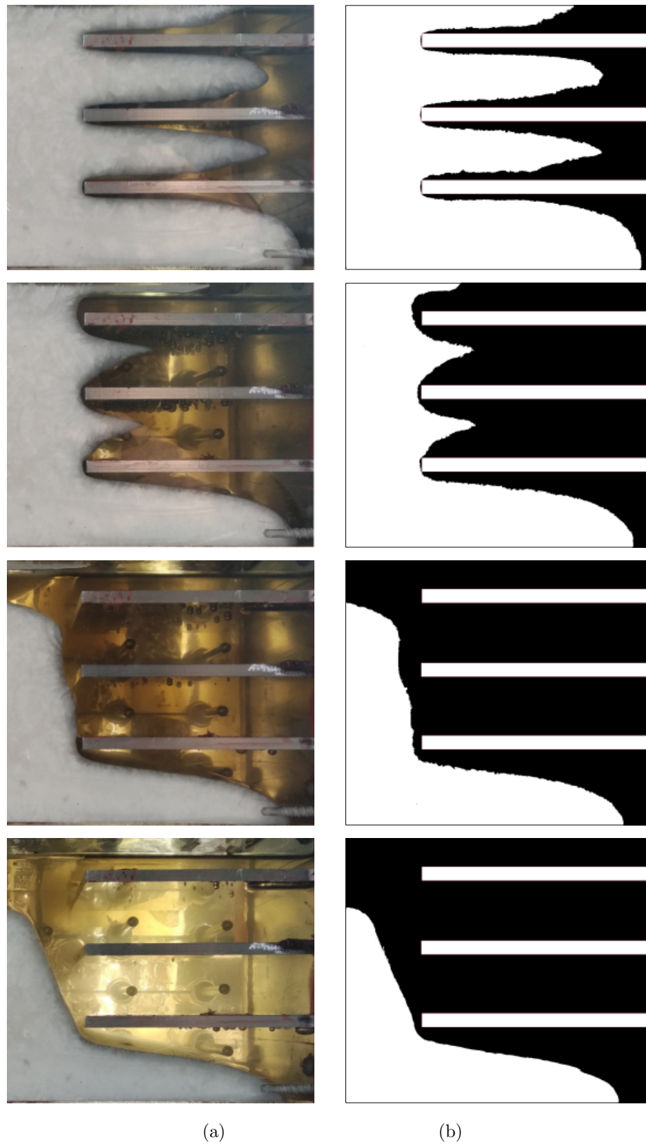
FIGURE 3.12: Melting front at different time steps (a) photographs and (b) digitally processed frames.
