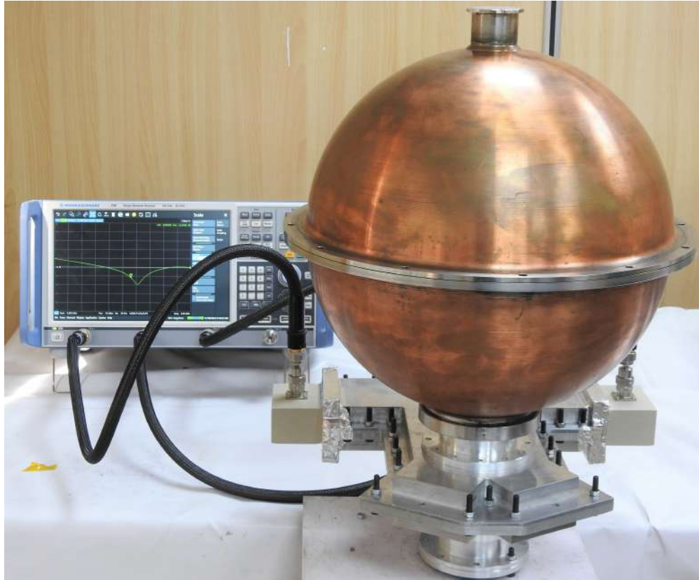
FIGURE 5.14: Pulse compressor assembly made from the copper cavity.
