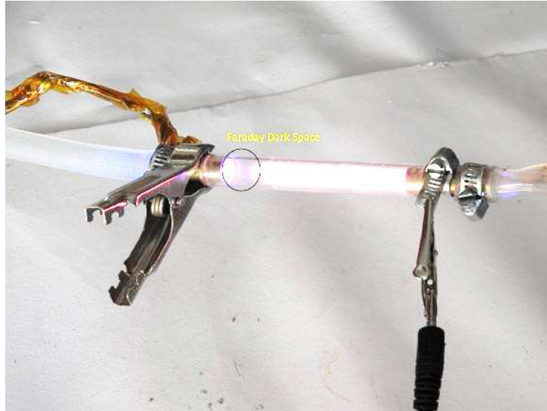
FIGURE 4.9: Experimental demonstration of DC glow discharge.
